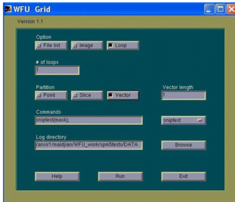
Figure 3. WFU Grid Distribution Tool. The user can choose the format of the input data (list of filenames, an image, or loop), the distribution partitioning scheme (point, slice, or vector), and the Matlab command to be distributed. All processing information is stored in the Log Directory
